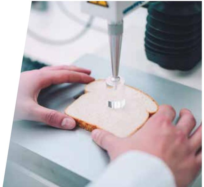
The compression test, during which a set force is applied for a certain time (phase 2), is used to measure crumb texture, especially its firmness  $F$  and elasticity ( $F'/F$ ).
