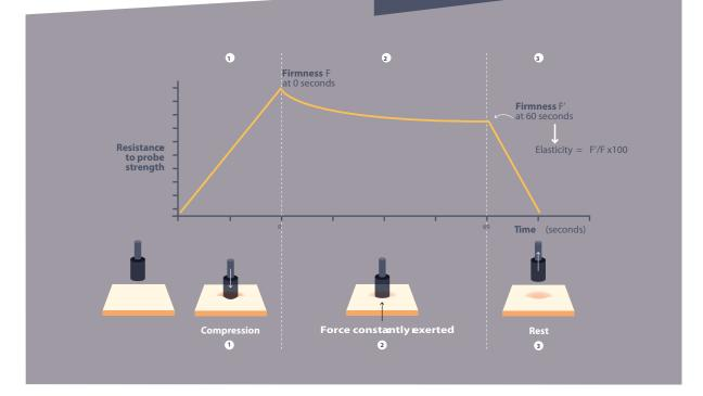
INSTRUMENTAL MEASUREMENT OF RESISTANCE TO CRUMB DEFORMATION (TEXTUROMETER)
