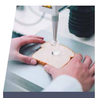
The compression test, during which a set force is applied for a certain time (phase 2), is used to measure crumb texture, especially its firmness F and elasticity (F/F').
