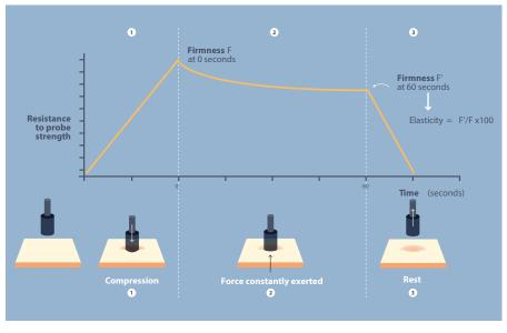
Figure 3. Principle of instrumental measurement of the crumb's resistance to deformation (texturometre).
